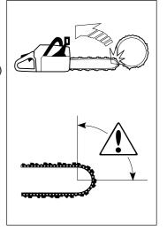
Kickback always occurs in the cutting plane of the saw. Normally the saw and bar are thrown backwards and upwards towards the user. However the saw may move in a different direction depending on the way it was being used when the kickback zone of the bar touched the object.
